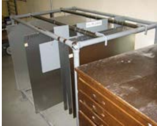
Fig. 2-5: Plates in queue on hanging rack in Press Room.
