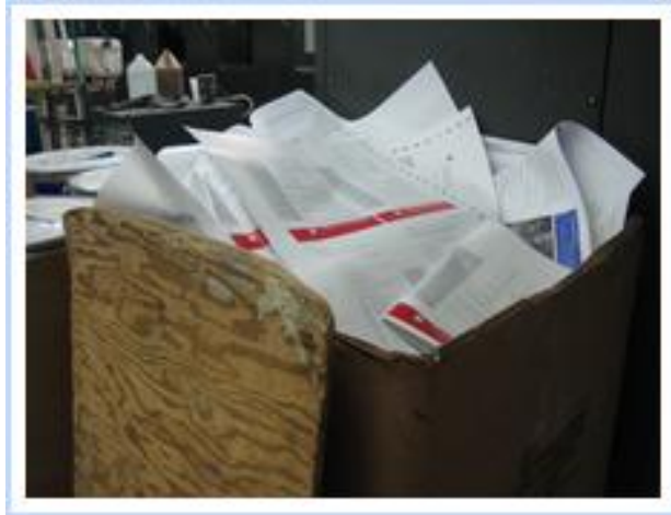
Fig. 2-6: Large amounts of scrap accumulate on shop floor due to Overproduction waste.
