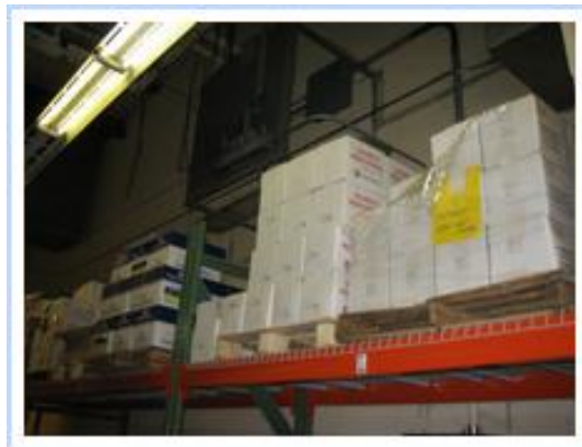
Fig. 2-19: Outdated finished goods inventory occupy vertical storage racks, causing current orders to be stored on the warehouse floor.
