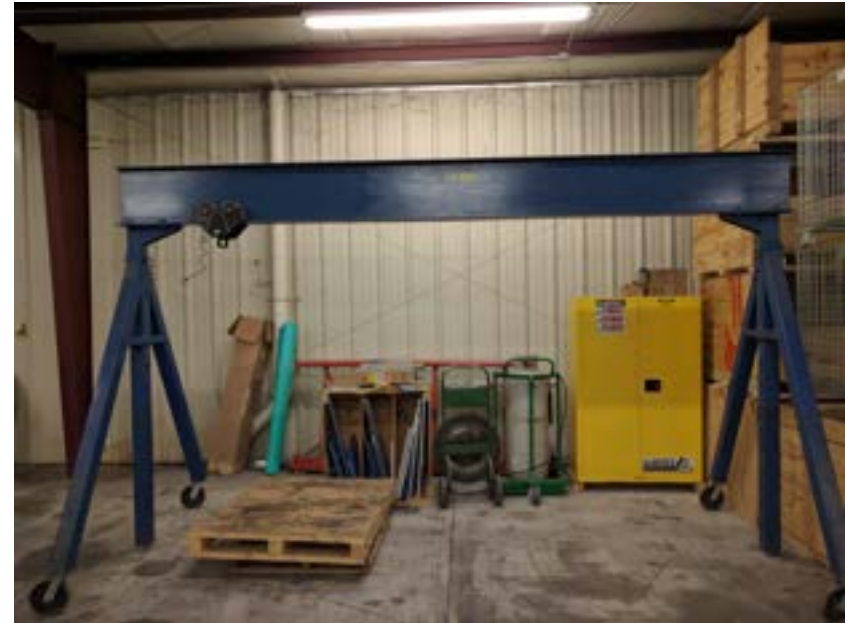
Temporary A-frame hoist
