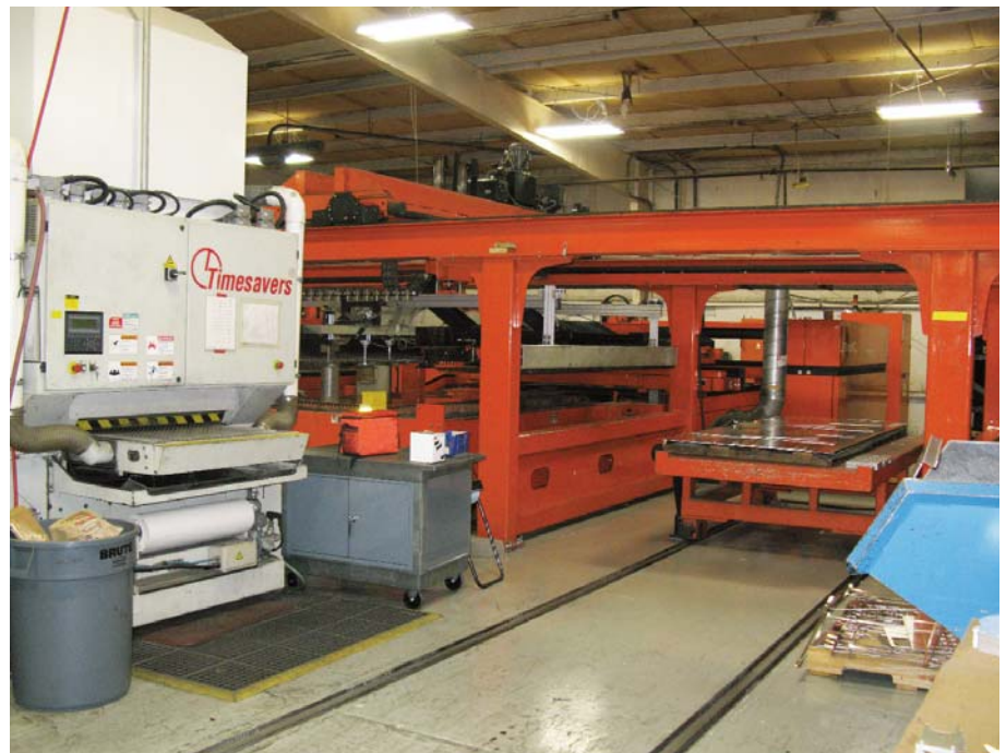
FIGURE 2 The company's laser cell includes a nearby deburring machine and (out of shot) a hardware-insertion press.
