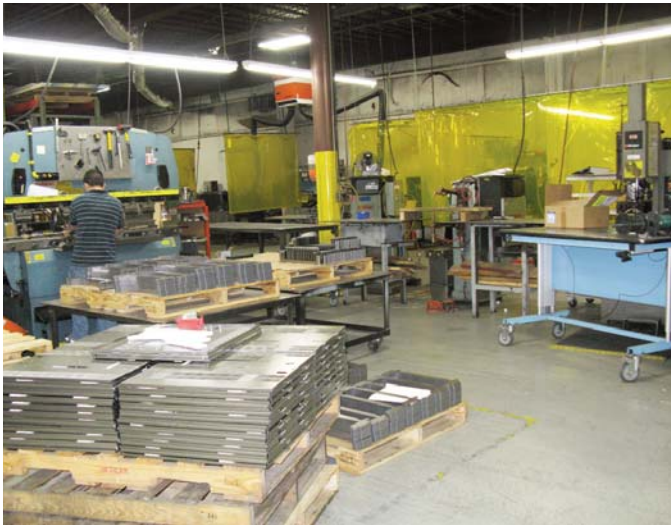
FIGURE 3 This cell has two press brakes, a hardware-insertion press (on the right), and a punch press (out of shot). The parts shown here have been punched and bent.
