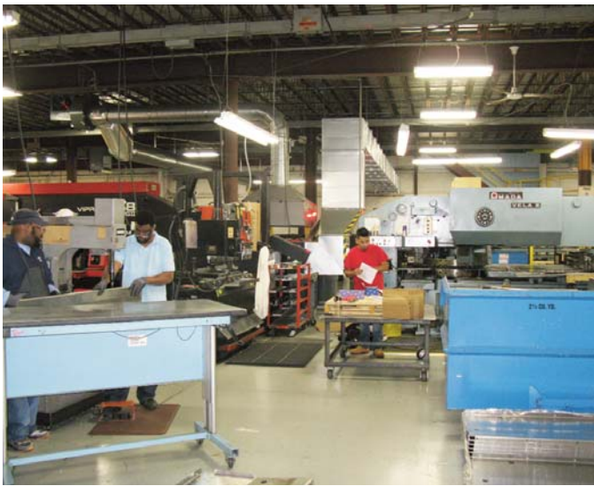
FIGURE 4 In this cell, two workers handle a panel for hardware insertion. Several minutes before, one worker at the hardware-insertion press was finishing a job at the press brake.
